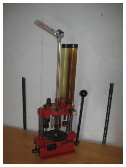
Hornady 366 Progressive Shot Shell Reloading Press. Cleaned and lubricated, replaced ball bearings with new and new primer tube filler mechanism.
