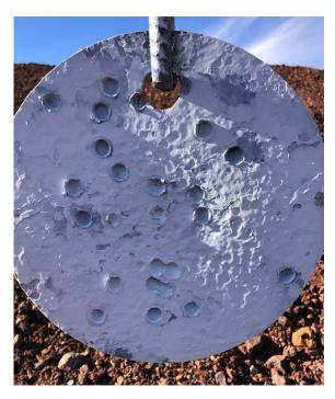
Last week an RSO discovered both gongs on the pistol section of the main range severely cratered. Someone with a .223 rifle did this. The gongs on the pistol side are not rifle rated!
